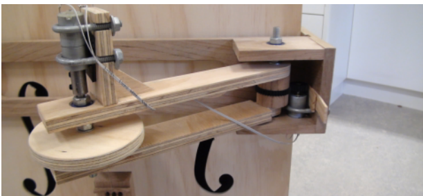
Fig. 2. First bowing mechanism and instrument design
